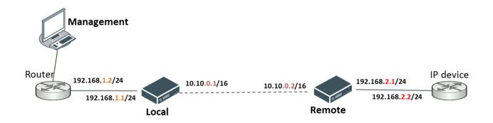
Different IP subnet L3 PTP Wireless Link - single IP subnet Different IP subnet
