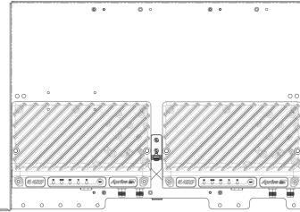
The Aprisa SR+ Data Driven Protected Station has an earth connection point on the left top of each radio. Use the supplied M4 screw to earth the enclosure to a protection earth.
