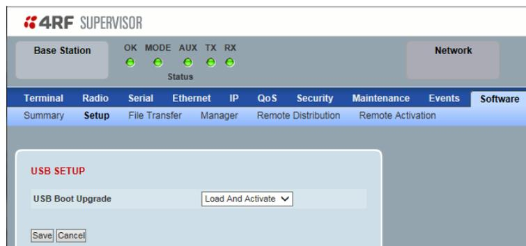
3. Power off the Aprisa SR+ and insert the USB flash drive into the host port
