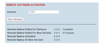
The remote stations will be polled to determine which radios require activation:
